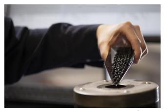
The recycled flame-retardant plastic Seculene® in the testing laboratory. Image: Ecobat
